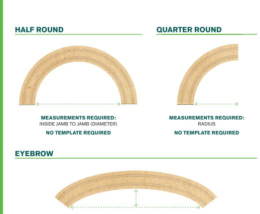
MEASUREMENTS REQUIRED: INSIDE JAMB TO JAMB AND RISE NO TEMPLATE REQUIRED
